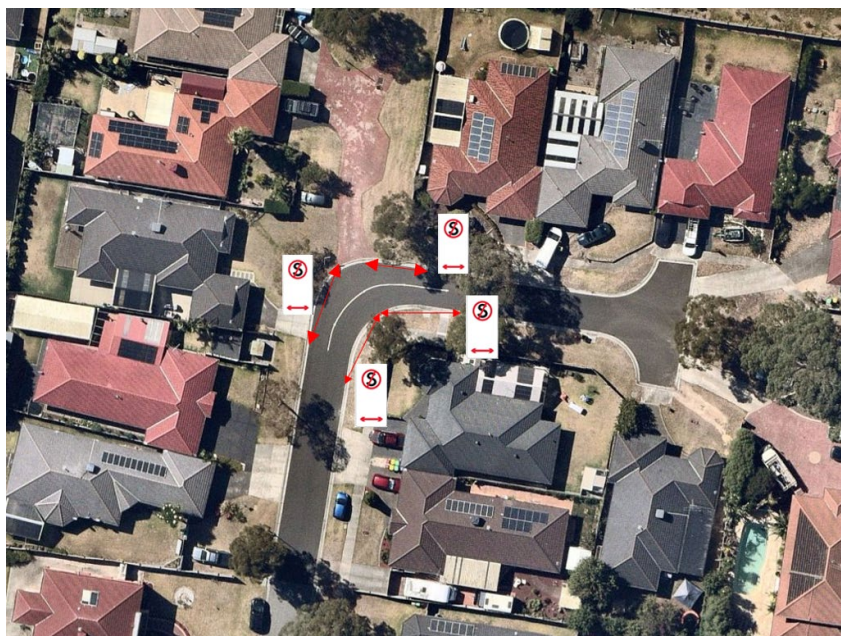
Figure 21 Approximate locations of 'No Stopping' signage along the bend (source: Nearthmap)
