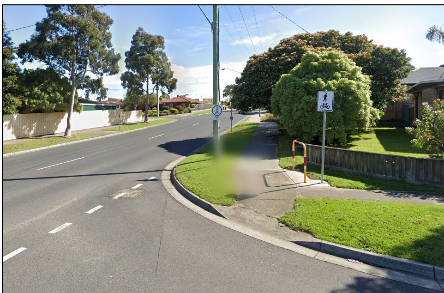
Figure 18 Tree blocking sight lines at intersection of Heysen Drive and McCormicks Road
