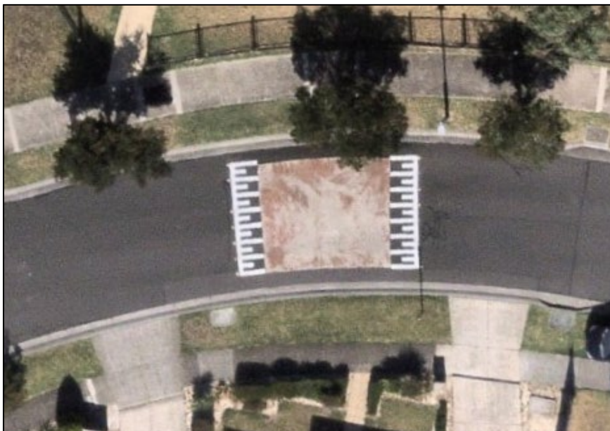
Figure 7 Example of a speed hump (source: Nearmap)
